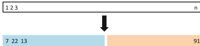
FIGURE 5.1. A schematic display of the validation set approach. A set of n observations are randomly split into a training set (shown in blue, containing observations 7, 22, and 13, among others) and a validation set (shown in beige, and containing observation 91, among others). The statistical learning method is fit on the training set, and its performance is evaluated on the validation set.
